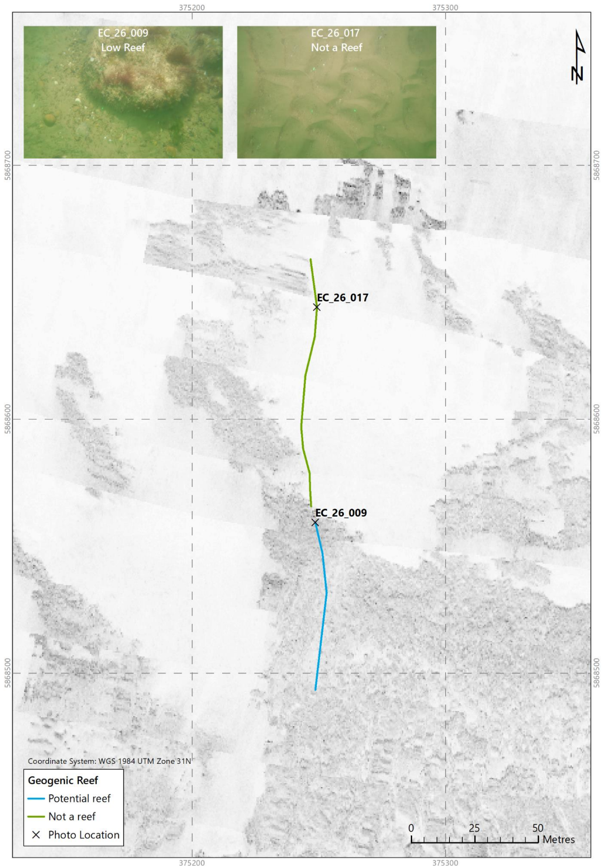
Figure 4.10: Potential geogenic reef (chalk) overlain on side scan sonar mosaic, transect EC_26
